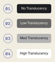
Translucency is critical for the *Charging Halo* to project light through stone and indicate the charging area.
